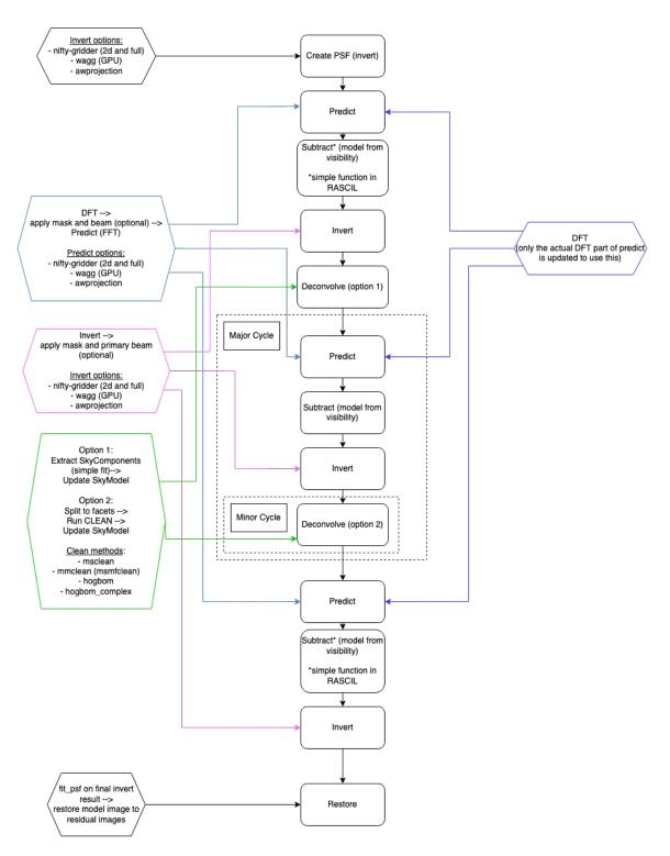
Currently, this structure is implemented using the *ContinuumImagingPipeline* class and tha main function in imaging\_prototype.py.
